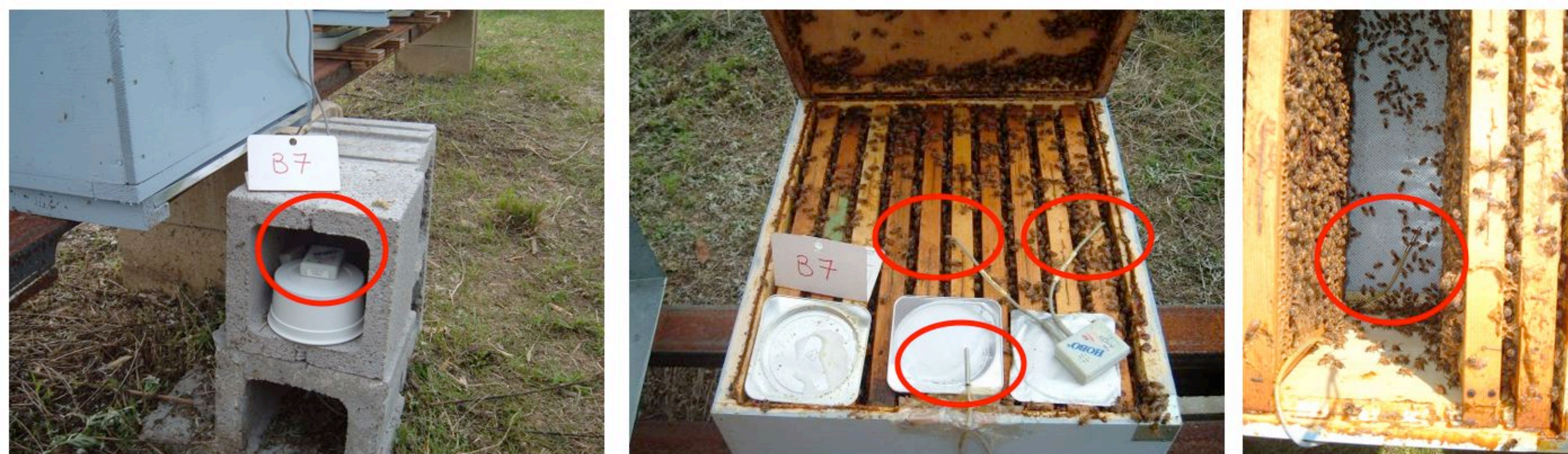
Figure 1. Data logger and temperature sensors placed inside the beehive on the honeycombs, on the beehive base, between the brood frames and between the last honeycomb and the lateral wall of the beehive
